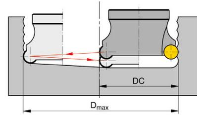
$D_{max.}$  = Maximum hole diameter Depending on the tool diameter
